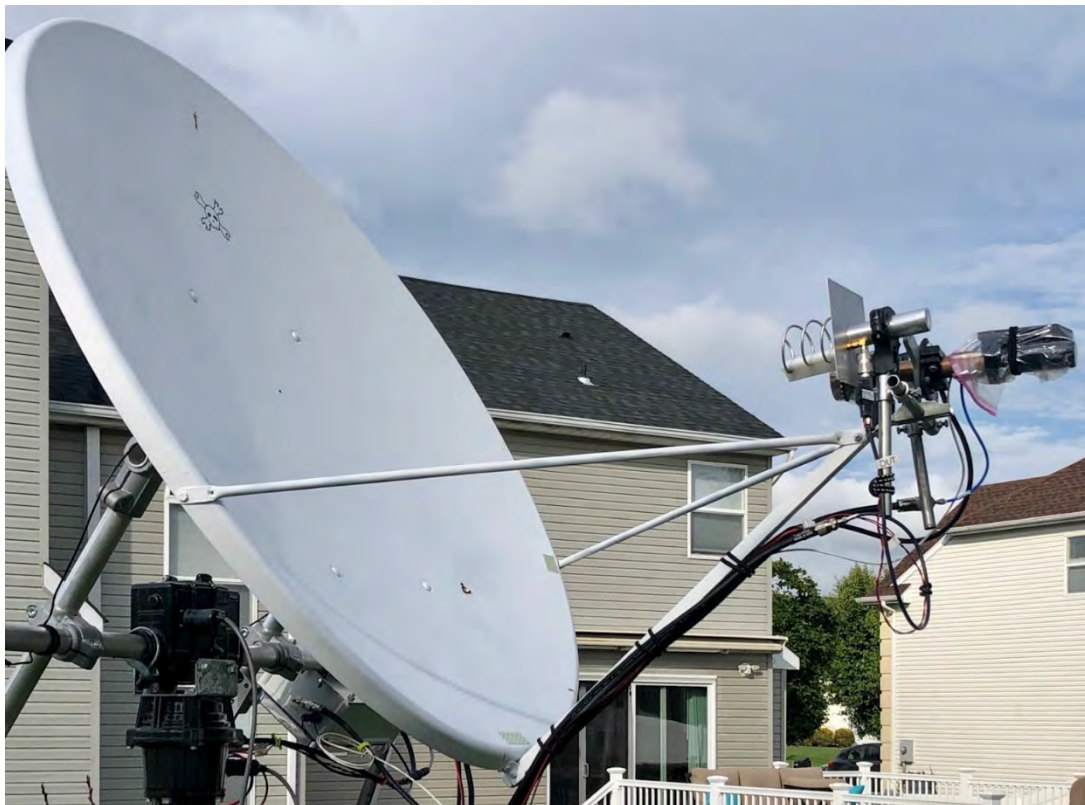
Figure 2 – Fortec Star 1.2m, f/d=0.6 offset dish shown with S-, X-, and Ku-band feeds
