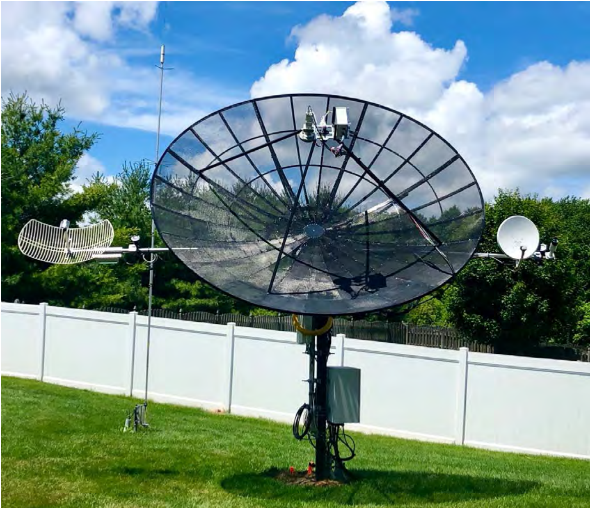
Figure 4 – 3.5m mesh dish with X-band feed and N2QG downconverter mounted on the feed-point bracket.
