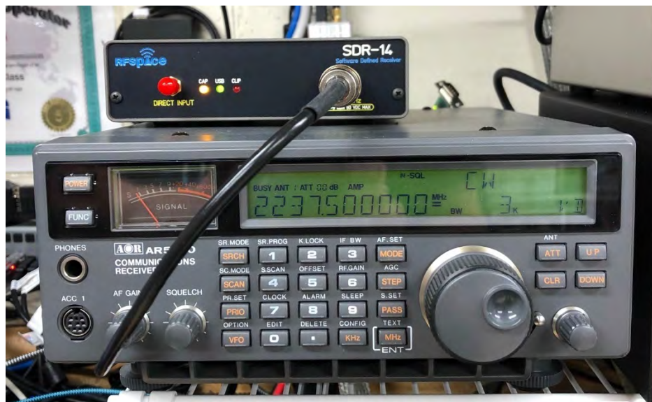
Figure 16 – My AOR AR-5000 receiver and the RFspace SDR-14 that I use for IF sampling.
