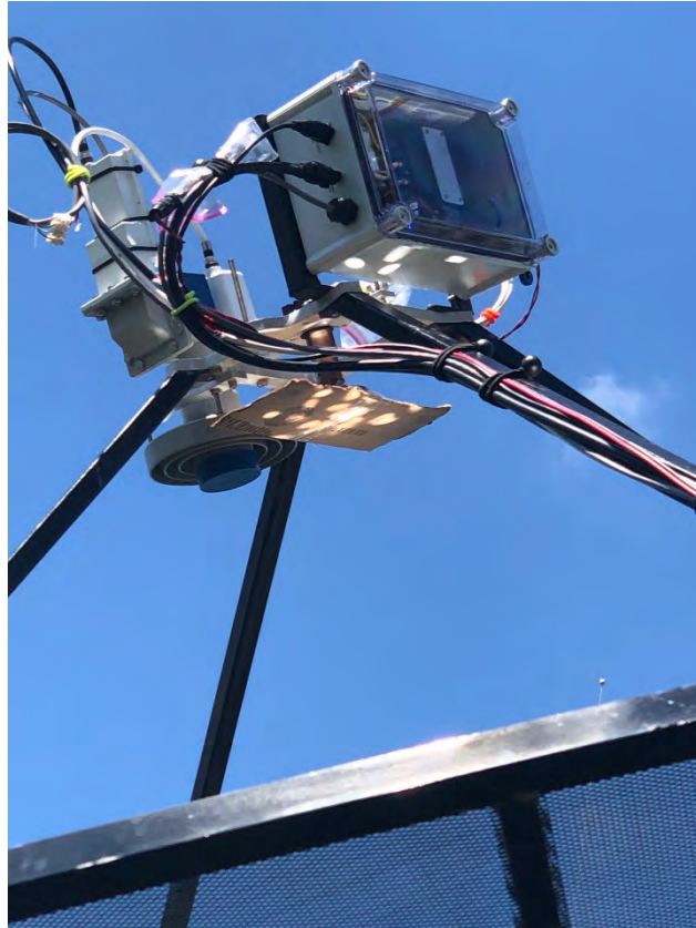
Figure 7 – Evaluating surface accuracy with small mirrors attached to the reflector shows spread at the focal point.
