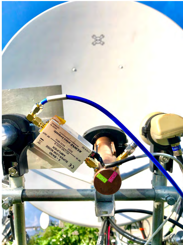
Figure 10 – Squeeze-tube depolarizer feed built by MOEYT. RHCP and LHCP probes added by KC2TDS.
