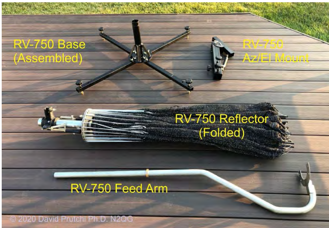
Figure 9 – Components of the EchoStar RV-750 collapsible antenna. Top: base and Az/EI mount. Center: folded reflector. Bottom: Feed arm.
