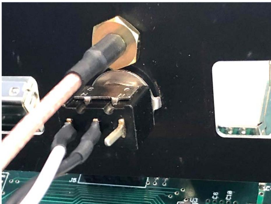
Figure 3 – A switch and a SMA pigtail need to be added to the back panel
