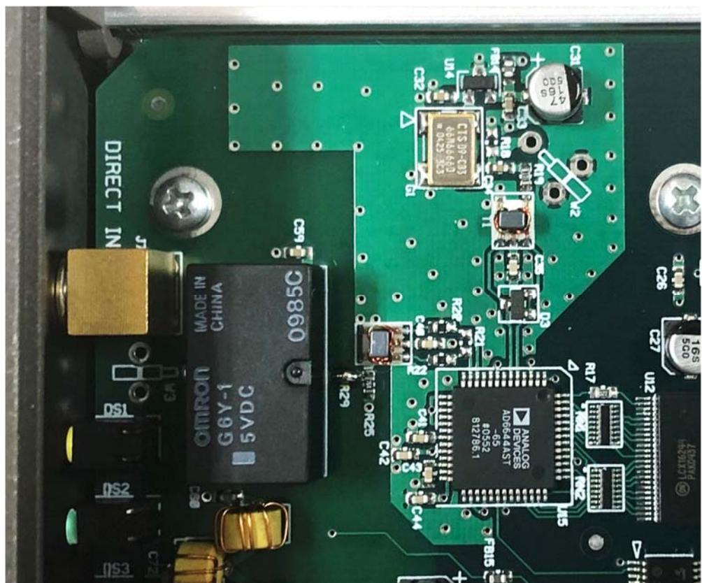
Figure 2 – Clock generator section showing G1 – the internal 66.666 MHz oscillator and W2 where the external source will be injected
