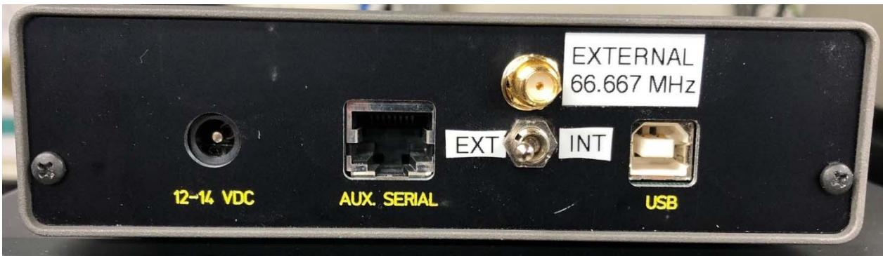
Figure 5 – Modified back panel of the RFspace SDR-14.
