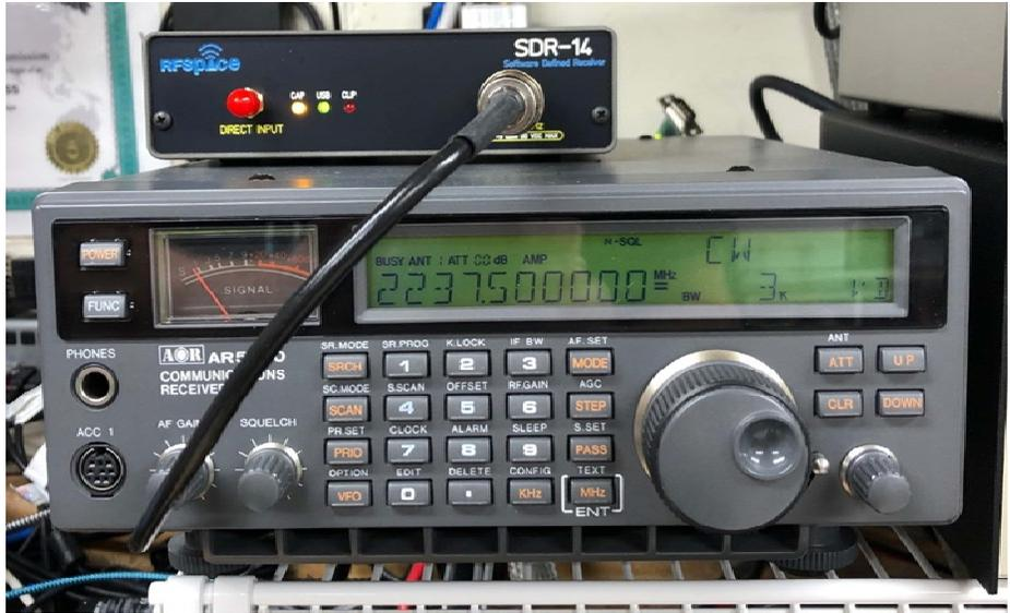
Figure 8 – AOR AR5000 and SDR-14 are now both GPS-locked for rock-solid frequency stability for EME and DSN RX
