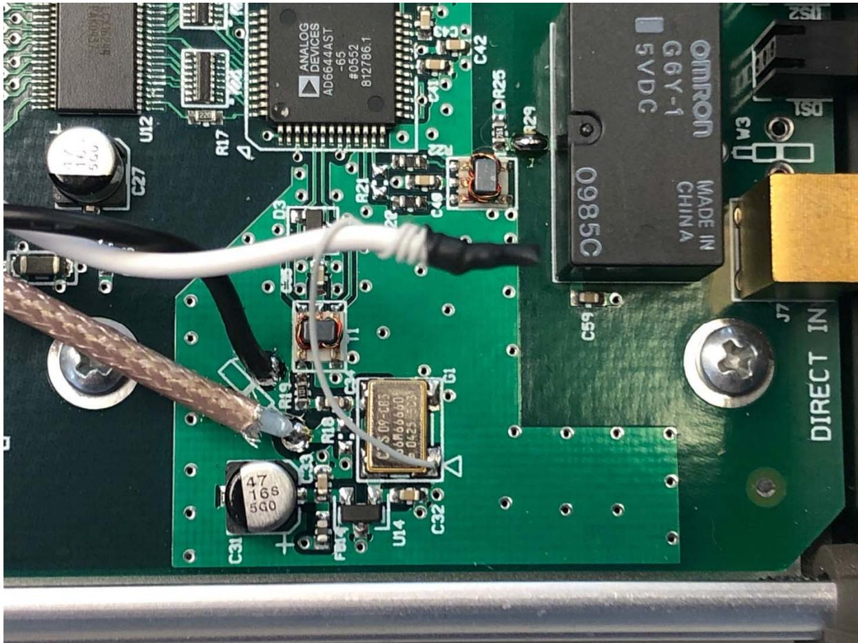
Figure 4 – The switch is used to turn off the internal oscillator when an external reference is injected via W2. The switch grounds pin 1 of G1 (identified by a triangle) to disable the internal oscillator.
