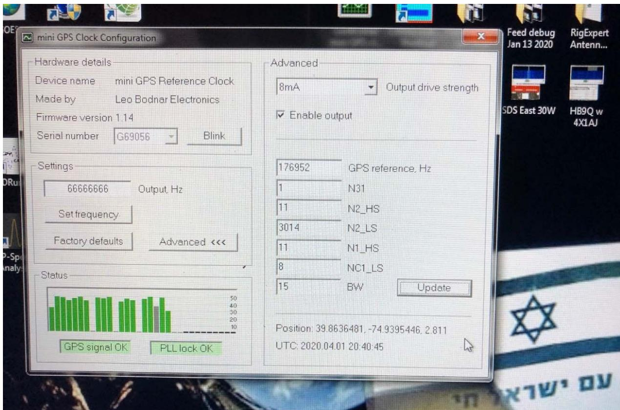
Figure 7 – The Leo Bodnar Mini Precision GPS Reference Clock needs to be correctly set up using its configuration software.
