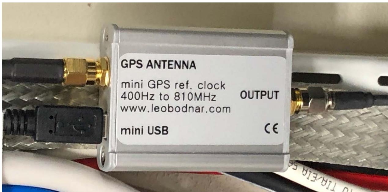
Figure 6 – I connected the output of a Leo Bodnar Mini Precision GPS Reference Clock to the new External Reference input to the RFspace SDR-14
