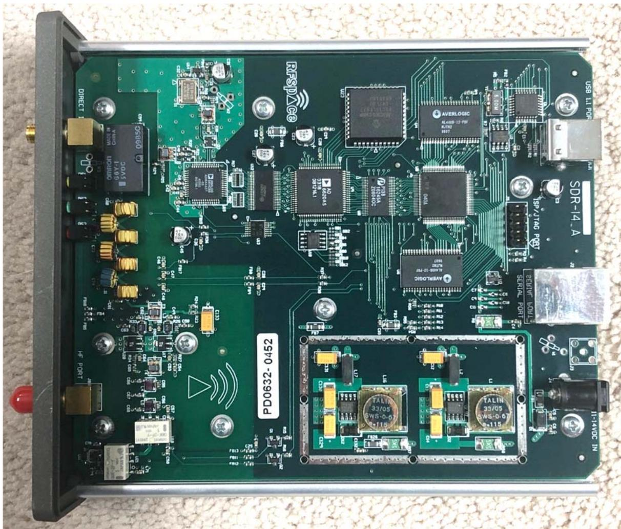
Figure 1 – Inside of the RFspace SDR-14. The internal clock generator is in the upper left corner of the PCB.
