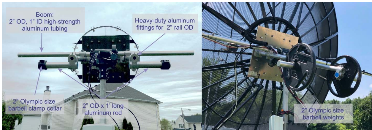
Figure 7 – My antenna is set up so that I can add Olympic-size barbell plates as counterweights. The weight plates are locked in place using barbell clamp collars, allowing me to quickly adjust the counterweight depending on the feed package installed at the focal point.
