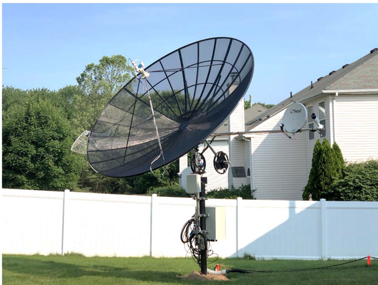
Figure 1 – Current status of my 12 ft dish for EME and amateur DSN. The boom also carries a GOES-16 antenna, a small Ku TVRO dish used to verify az/el calibration, and a high-resolution TV camera to show me at what the antenna is pointing.
