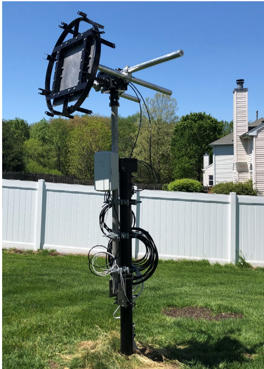
Figure 6 – The boom and dish arms are made of 2" OD, 1" ID high-strength aluminum tubing
