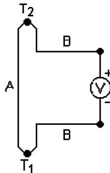
**Figure 2** – In a thermocouple, a voltage - the thermoelectric EMF - is created in the presence of a temperature difference between two different metals or semiconductors. In the isotopic thermoelectric generator, many thermocouples are arranged in series/parallel to form a thermopile which produces useful power levels. One of the junctions of each thermocouple (e.g. T1) is exposed to the heat generated by the decay of the Pu-238, the other junction (e.g. T2) is at body temperature.
